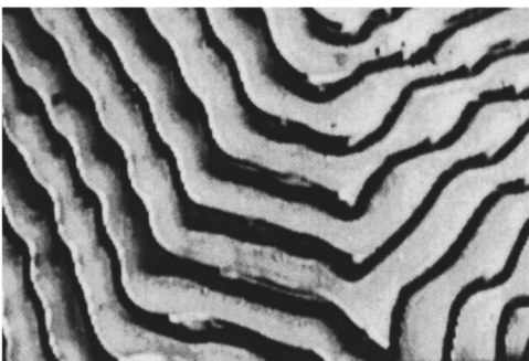
FIG. 10. The VRL transverse instability. The transverse instability shown in this photo is rather weak, and has a clear direction of orientation. The left part of VRL which is perpendicular to this direction is affected most. The shape of the VRL is determined by the boundary. A more typical VRL TI can be found in [1,9]. Sample thickness d = 40 \mu\text{m} .
