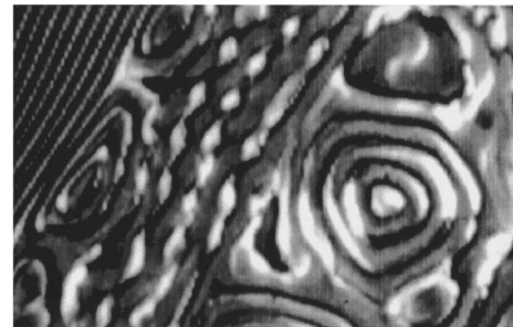
FIG. 12. The short-wavelength lattice is seen at the top left corner. It is growing into the complex region. Sample thickness d = 100 \mu\text{m} .
